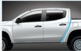
The J-line design is a clever engineering design made to shorten the wheelbase and maximize interior space.
